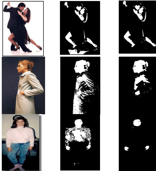
FIGURE 2: Comparison between pixel-based [2] and region-based skin color classification techniques. Left column shows the original images. Middle column shows the result of pixel-based classification technique and right column shows the result of region-based classification technique with CRF.
